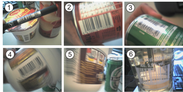
Figure 3. Recognition conditions: 1. Small code, 2. Unsharp image, 3. Reflections, 4. Fuzziness due to rotation, 5. Code movements, 6. Difficult lightning conditions
